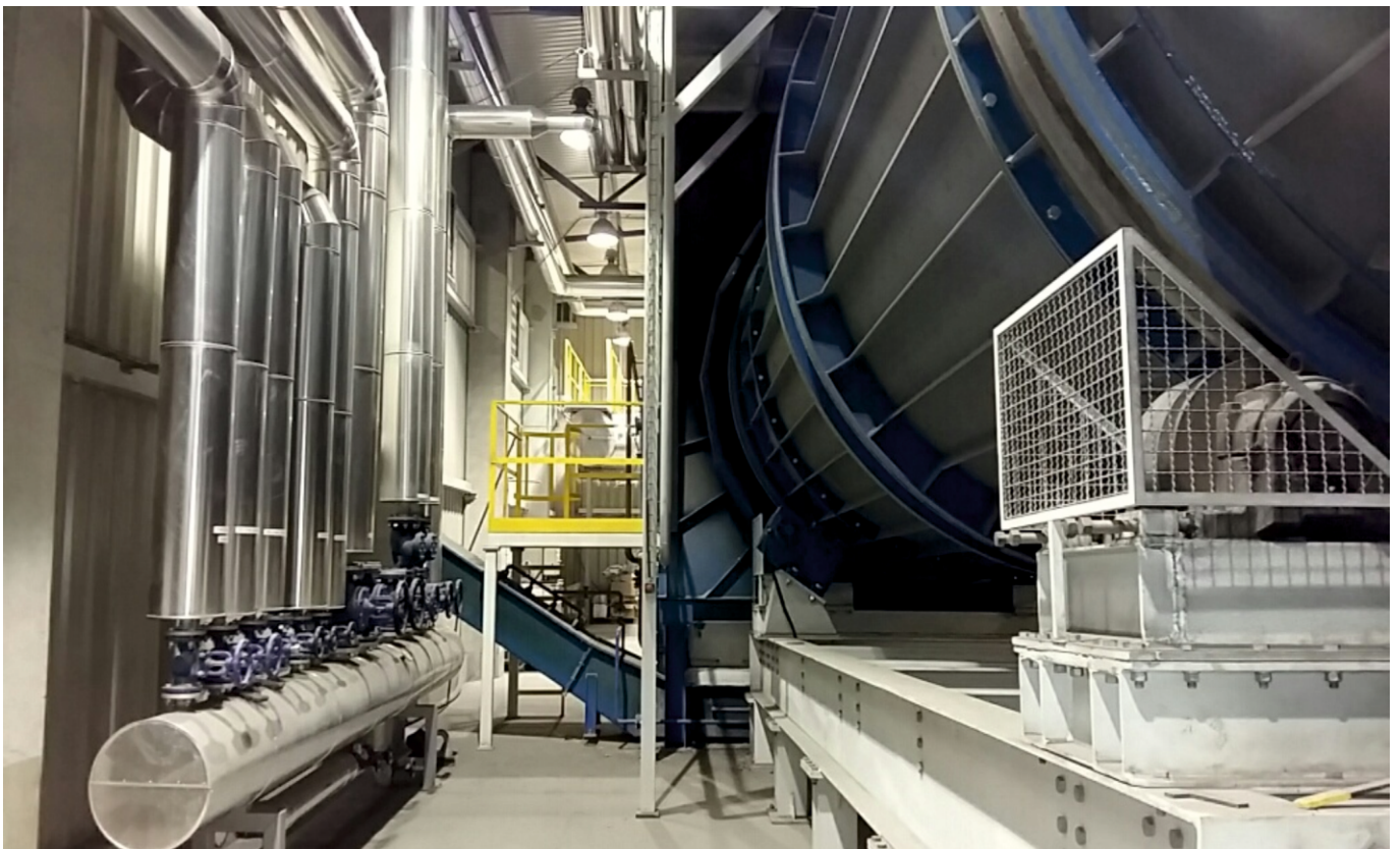
ROTARY KILN WITH A CAPACITY OF 1250 kg/h
